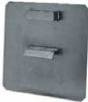
Lightweight, totally aluminum board constructed with "L" shaped bracket on back that slips over the top of the form. Naturally helps reduce spillage and removal of form oil off forms at discharge locations. Directs uniform flow of concrete during placement.
